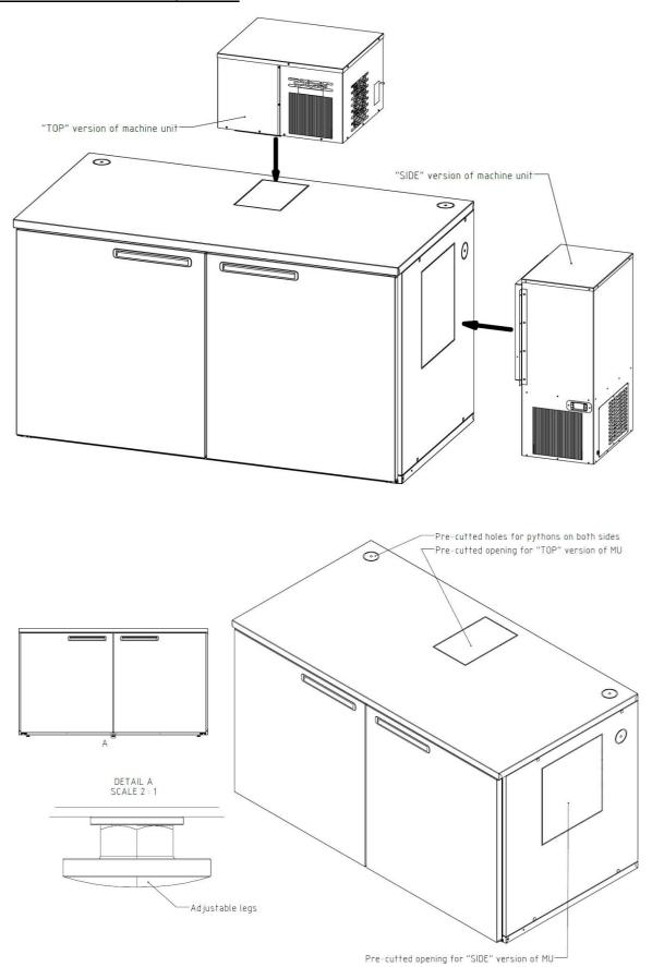
Cooling equipments are equipped with exterior and interior from sheet coated by plastics, adjustable legs, digital thermostat, air cooling.
