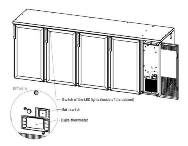
Cooling equipments are equipped with shelves, drawers, bottle holders, exterior and interior from sheet coated by plastics, adjustable legs, digital thermostat, air cooling, interior illumination and some of them have door locks
